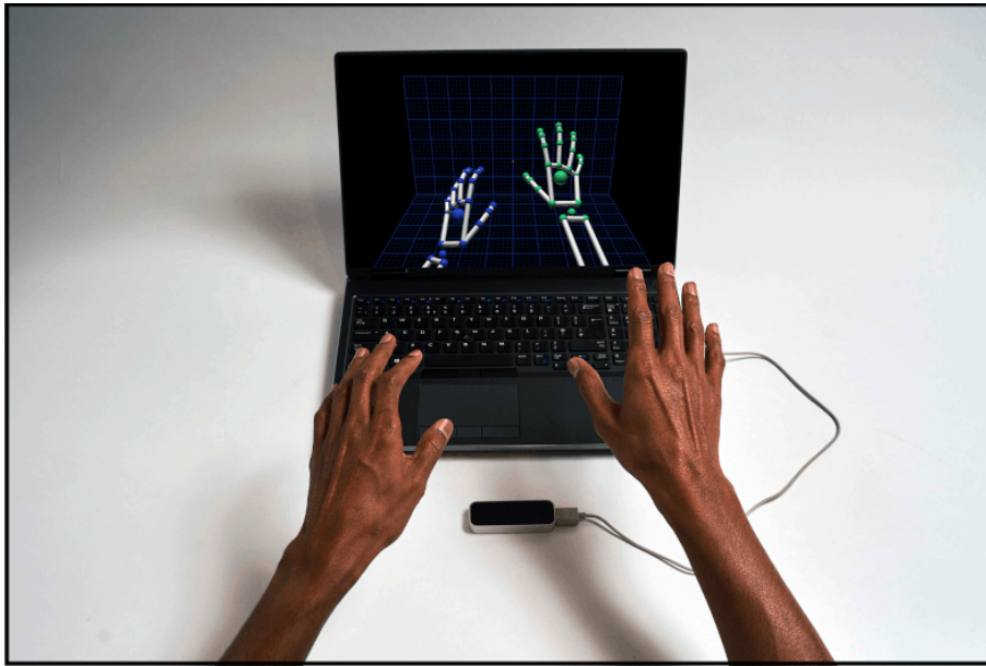
Figure 1.6: This figure presents the Leap Motion Controller device and illustrates the human-computer interaction style supported by the technology. The image was retrieved from the Ultraleap website [8].
