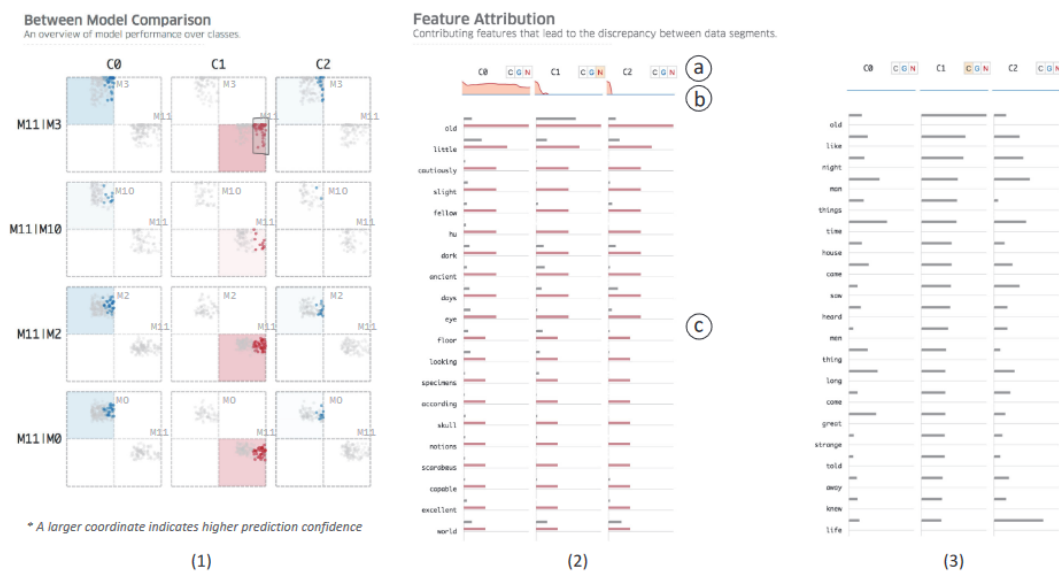
Figure 2.8: Manifold main views [59]. This VA tool includes the model comparison overview in (1), which provides a visual comparison of pairs of models using a small multiple design. The local feature interpreter view (2) which shows a feature-wise comparison between user-defined subsets, as visible in (c), and provides a measure of similarity between the feature distributions, see (b). In (a), the user can sort the features based on various metrics, and then in (3), it is possible to identify the most distinguishing features among different subsets or a specific class.
