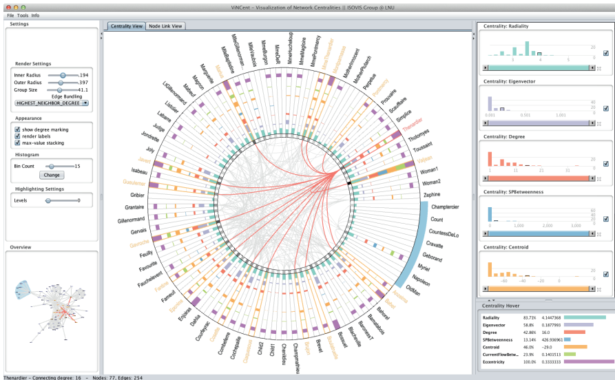
Figure 2.2: Overview of our network visualization tool ViNCent [96, 170]. The network is drawn as a circular view together with network centralities as bars. The right side displays the corresponding histograms of the network centralities as well as detailed values of the network centralities for the currently hovered node “Thenardier”. ©Linköping University Electronic Press.
