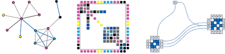
Figure 2.3: Three types of general graph visualization techniques: node-link diagram (left), adjacency matrix (middle), hybrid (right). Image taken from [76]. ©IEEE.
