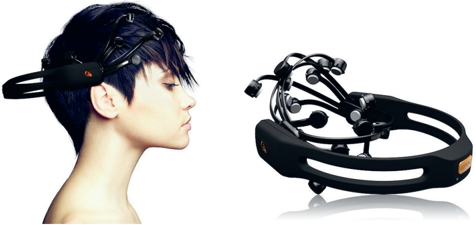
Figure 4.2: The Emotiv EPOC EEG headset (images courtesy of Emotiv).
