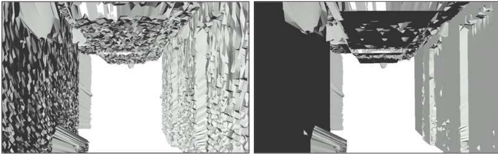
Figure 2.13: Mesh model from 3D point cloud of the Wean Hall at the Carnegie Mellon University (left) and equivalent smoother, low complexity mesh model obtained by planar approximation (right)
