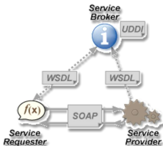
Figure 3.8. Web Service communication architecture
