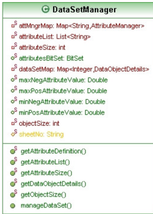
Figure A.8. DataSetManager: Class Design Diagram
