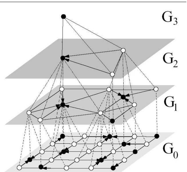
**Figure 1. A small graph pyramid based on a  $5 \times 5$  pixel image (taken from [6]).**
