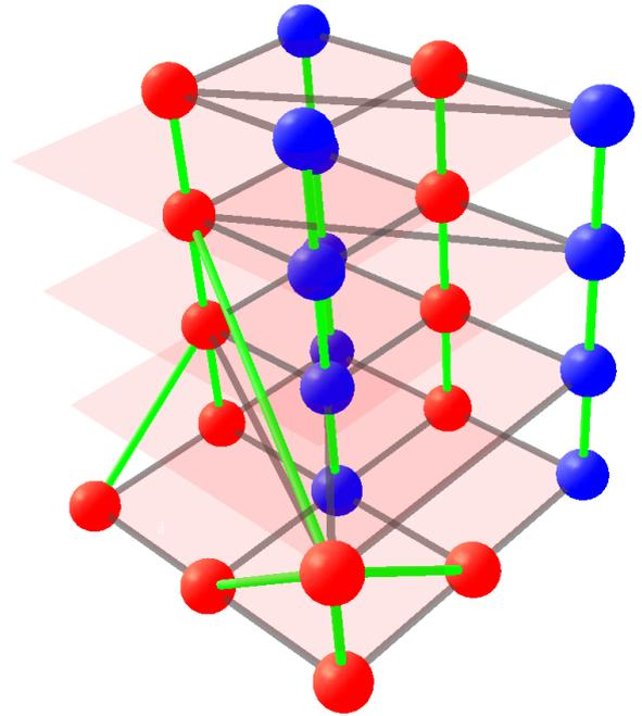
Figure 2. The graph pyramid of a  $3 \times 3$  pixel image.
