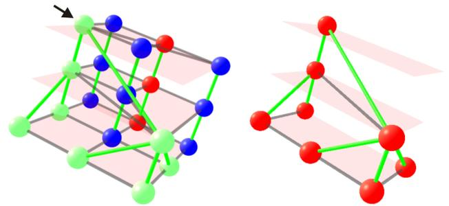
**Figure 7. The left picture shows a selection of one node. When the topmost green node is clicked (see black arrow), all of its subnodes are automatically selected as well. At the same time the selected subpyramid is drawn, which can be seen in the right picture.**
