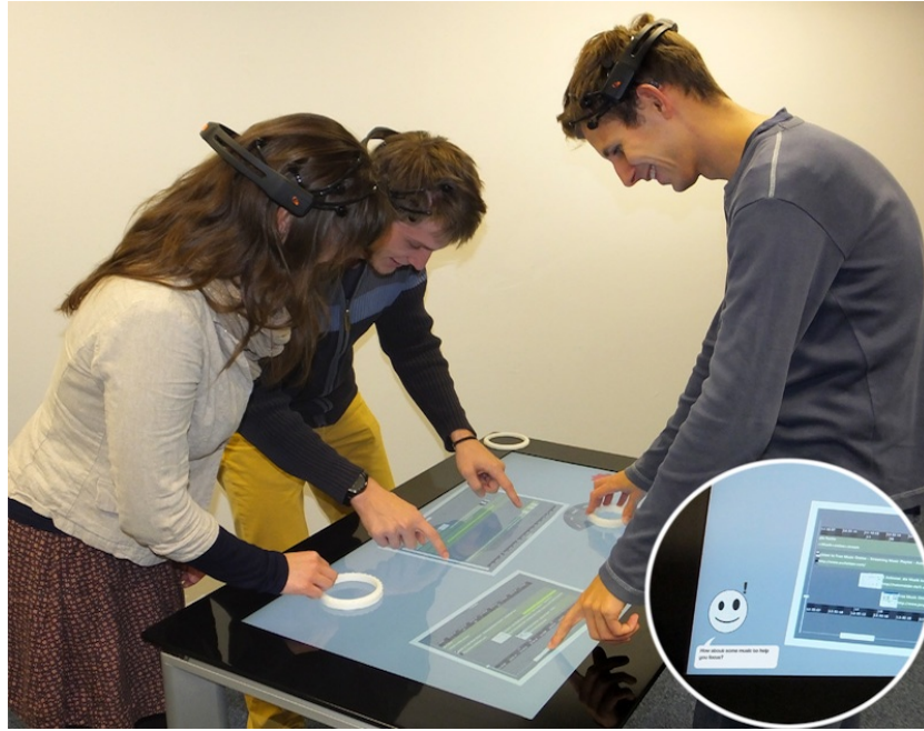
Fig. 3. Users collaborating around a tabletop application while wearing BCI devices that interpret their affective states. The GAT virtual agent inspects these affective states and offers real-time feedback about the group affective tone, as well as suggestions for developing a PGAT.
