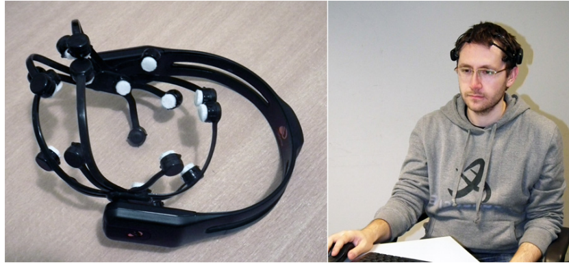
Fig. 1. Image of the Emotiv EEG neuroheadset (left). User wearing the EEG device while interacting with a computer (right).
